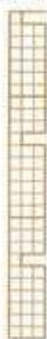
N – Horizontal Wall Support (cut 2, leaving single bar at end) 3 x 27 holes
