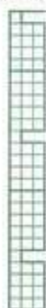
M – Horizontal Wall Support (cut 6, leaving single bar at end) 3 x 25 holes
